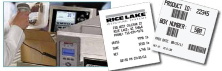
With two standard serial communication ports and 20 configurable custom print formats, designing custom labels and tickets to include logos, IDs, net weight, bar codes, and more is easy with the 820i.
